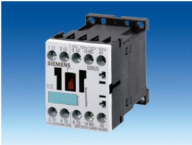
SCHUETZ, AC-3, 3KW/400V, 1S, DC 24V, 3POLIG, BGR. S00, SCHRAUBANSCHLUSS
